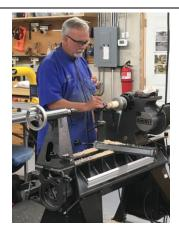
Tracy Casselman presented a demo on spinning tops. He used a 2"x 2"x 6" blank of hard maple which he rounded between centers using a spindle roughing gouge. He then made a tenon on one end and mounted it in a 4 jaw chuck. He turned one spinner, decorated it on the lathe using various colored markers, pens, etc. then parted it off and turned a second spinner from the same blank which he decorated with a chatter tool then colored with sharpie pens. Thanks Tracy!
