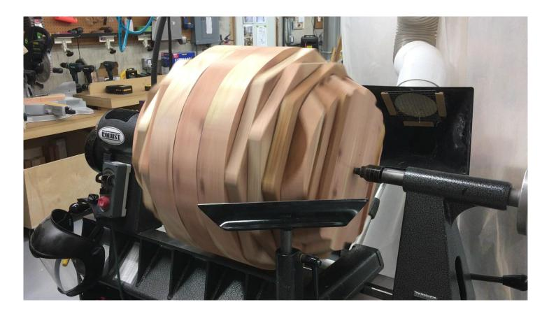
Luckily, it fit! There was about ½" clearance over the bed. We mounted it using a spur drive and a live center. The spur drive turned out to be a bad choice as the wood was so soft that when we slowed it down to stop, the piece would try to keep moving and tear out where the spur drive was. By the way, the only good way to stop a piece this big is to slowly dial the speed down as low as possible before turning the lathe off.
