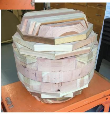
Now that the blank was complete, we put it on the lathe. It weighs about 75 lbs.
